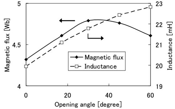
Fig. 9. Magnetic flux and inductance results.
