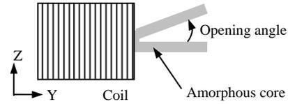
Fig. 8. Aperture angle of the amorphous metal core.
