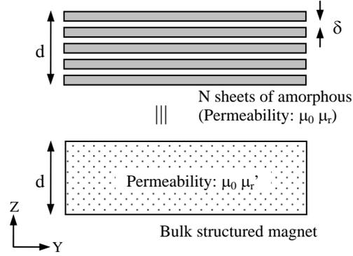
Fig. 7. The magnetic body with the equivalent bulk structure.
