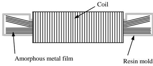
Fig. 6. Structure of amorphous metal core loop antenna.
