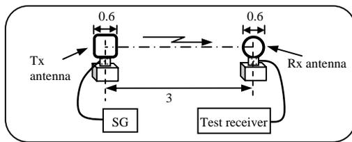
Fig. 2. Measurement setup using standard loop antenna.
