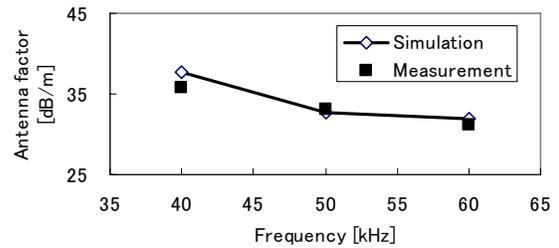
Fig. 5. Antenna factor of the MCLA.
