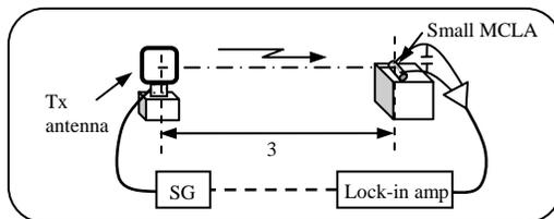
Fig. 3. Measurement setup using the MCLA.
