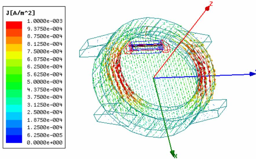
Fig. 10. Current density generated in a metal case.
