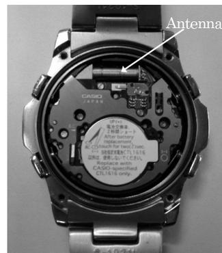
Fig. 13 The interior side of a radio controlled watch with an all-metal casing.
